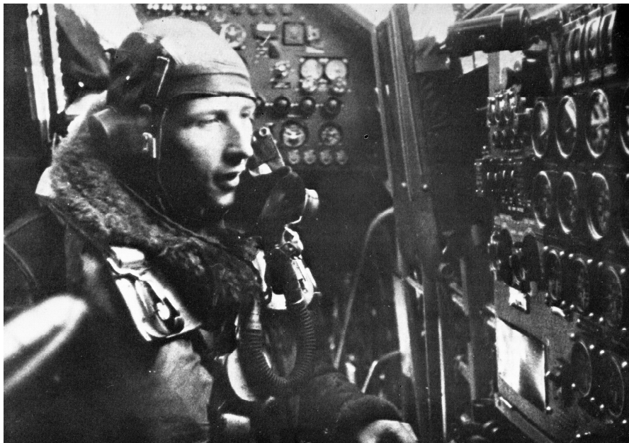
Lancaster Flight Engineer checks the instruments on his console The Second Dickey seat can be seen folded in its stowed position
