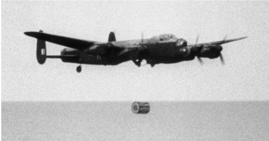
Successful Upkeep release at Reculver
