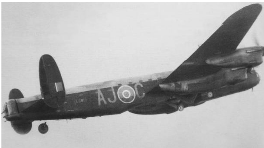
Avro Lancaster B.III (S) Type 464 - ED817 showing V-Shaped Callipers for holding the Upkeep
