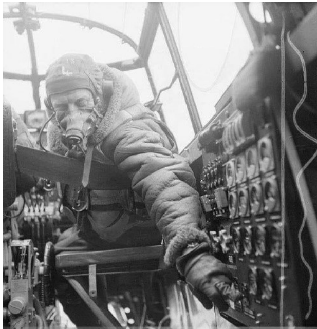
Lancaster Flight Engineer flicking the fuel contents switch to check fuel levels
